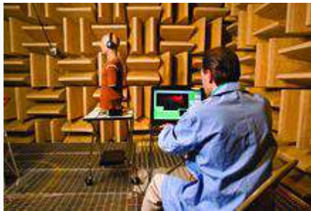
Example of safety product testing: headphones in anechoic chamber.
