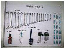
Shadow board (with tools' outline) and worker's movement that is being used in production floor
